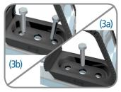
**3.** Secure cleat to the mounting surface using  $1 \times M10$  bolt (3a) or  $2 \times M10$  bolts (3b), adding a washing and nut on both sides.
